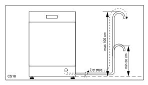
Likewise the internal diameter of the couplings used for connections to the waste outlet must be no smaller than the diameter of the hose provided.
